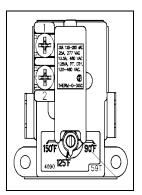
The lower thermostat performs the same basic function as the upper thermostat. It controls the flow of electricity to the lower heating element. When the water in the lower portion of the water heater becomes hot, the thermostat will open and stop the flow of electricity to the heating element. When the water cools to a temperature below the thermostat setting, the contacts close allowing electricity to flow to the heating elements.
