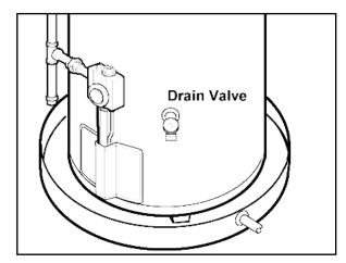
Use a new ¾ inch N.P.T drain valve Seal threads with Teflon tape of pipe sealer
